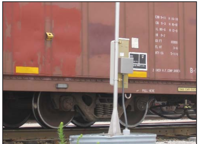
Scanners with antennas collect information from RFID tags on each train car.
