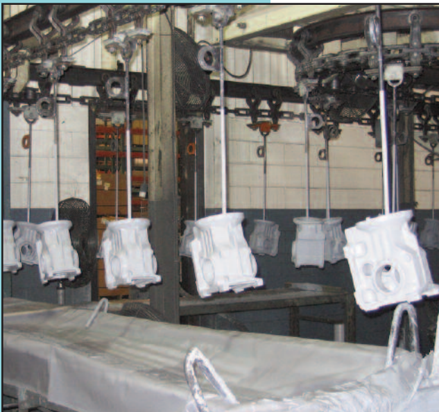
Gear boxes along the paint assembly line
