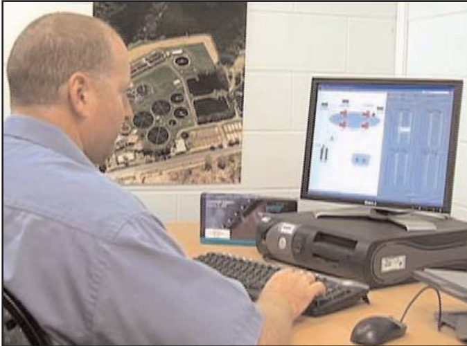
Plant operators can easily monitor and control equipment through the Wonderware InTouch human-machine interface
